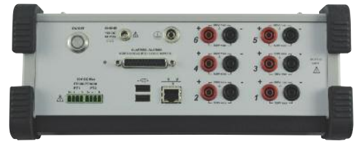
6 analogue isolated channels 2 Pt100 input and 16 logical channels.
