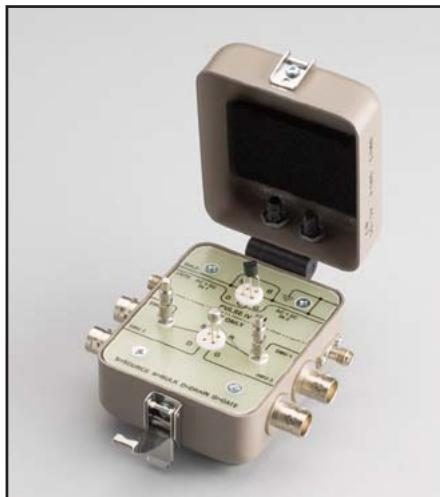
**Model 8101-PIV:** DC and pulse LV demo fixture that is a metal case with four female triax connectors, two SMA connectors, and a latch. Inside the test fixture are two 4-pin device holders (transistor sockets) and two plungers for parts with two leads.
