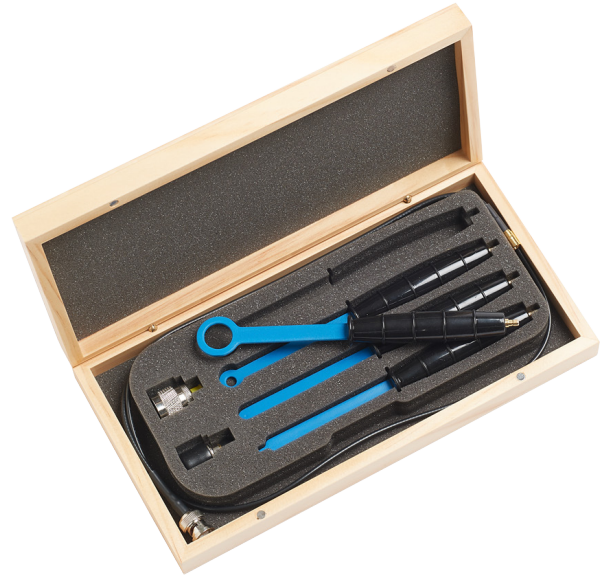
FIGURE 33. A near field probe can be used to discover the location of unintended RF emissions.
