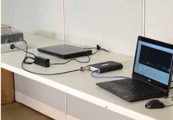
Figure 13. Basic pre-compliance conducted emissions test setup.
