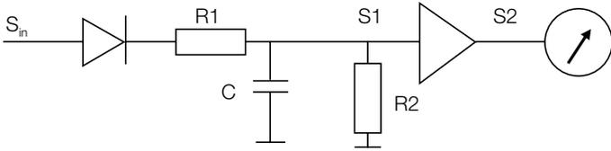
**Figure 5.** Quasi-peak detector in an analog implementation. The fast-attack (charge time) and slow-decay (discharge time) of the quasi-peak detector result from the R-C constants implemented in this circuit. The resultant waveform drives the critically-damped meter.
