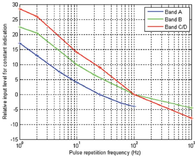
**Figure 7.** Pulse response curve with a Quasi-peak detector.
