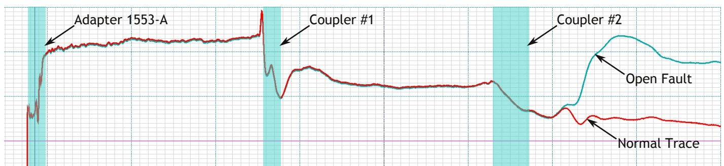
Figure 3: MIL-STD-1553B main bus open conductor fault detected through two transformer couplers using adapter 1553-A. The transformer regions of the TDR waveform are shown in shaded blue boxes.
