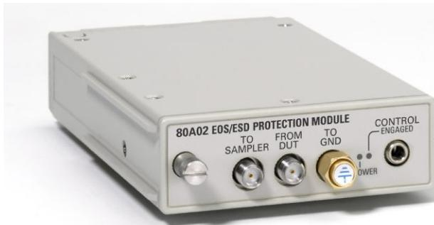
The 80A02 EOS/ESD Isolation module protects the sampling bridge of Tektronix DSA8300<sup>1</sup> electrical sampling module inputs from damage due to electro-overstress (EOS) and electrostatic discharge (ESD) from circuit boards and cables. The 80A02 is for applications such as electrical TDR circuit board testing and cable testing where large static charges can be stored in the DUT.
