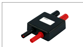
989006000 : 1 ohm shunt, 0.1%, 0.5A max
