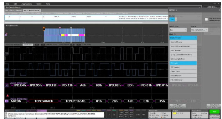
Automotive Ethernet Protocol Decode for full-duplex ECU
