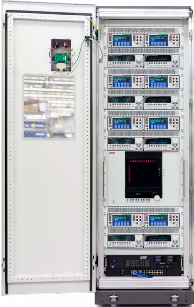
Figure 7: Typical test rack with multichannel high accuracy DMMs and related switching unit
