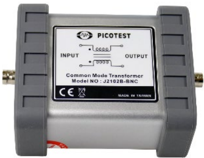
The Picotest J2102B works with the probe to break the inherent ground loop present in the 2-port shunt-through test.
