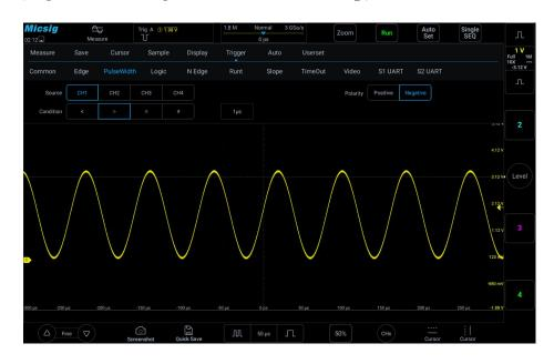
Figure 6-15 Negative Polarity Pulse Level Flip
