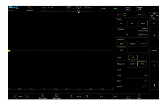
Figure 5-9 GND Coupling
