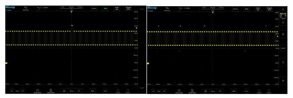
Figure 6-3 Abnormal Signal in Periodic Signals
