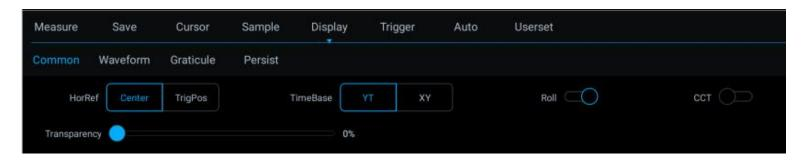
Figure 10-1 Display Settings and Function Buttons
