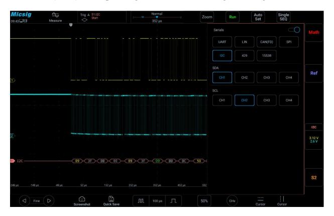
Figure 12-22 I<sup>2</sup>C Bus Configuration Menu
