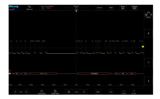
Figure 12-16 CAN bus decode interface
