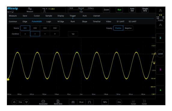
Figure 6-14 Pulse Width Trigger Setting Menu
