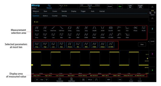
Figure 7-1 Automatic Measurement Menu
