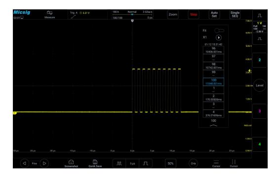
Figure 11-12 Segmented storage single frame viewing
