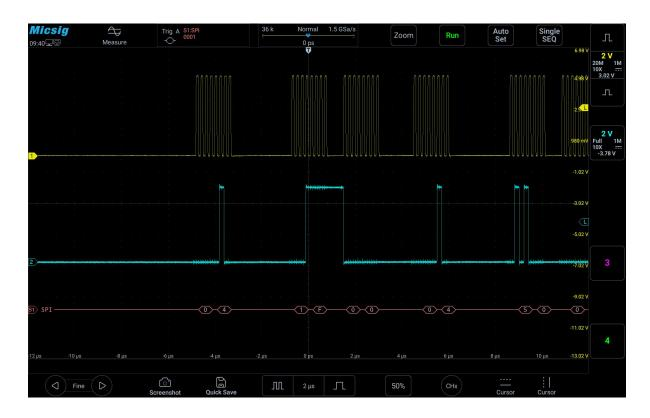
Figure 12-20 SPI bus decode interface
