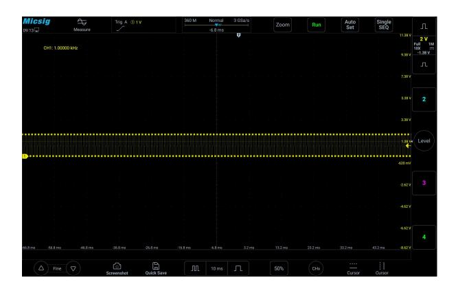
Figure 7-15 Frequency Meter Measurement
