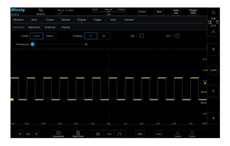
Figure 10-5 Color Temperature Open Mode
