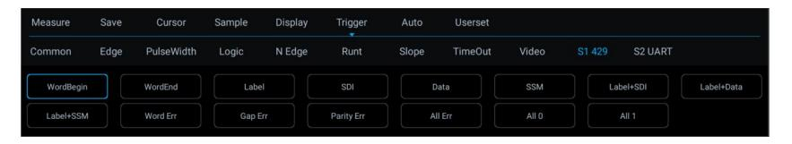
Figure 12-27 ARINC429 Trigger Mode Configuration Menu
