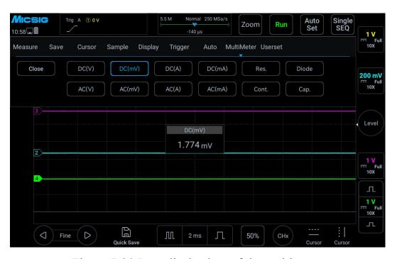
Figure 7-20 Data display box of the multimeter
