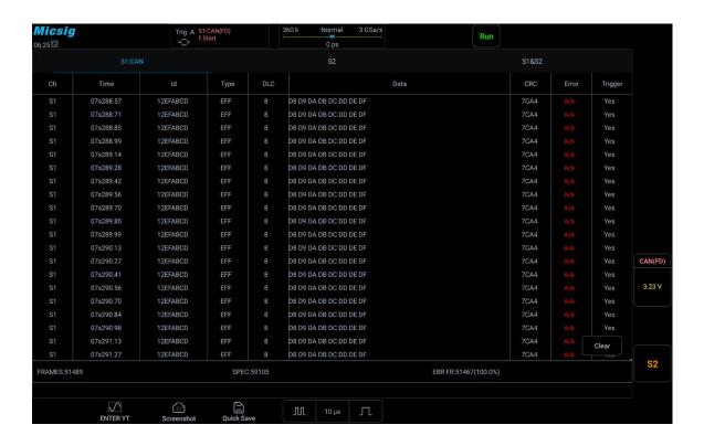
Figure 12-17 CAN bus decode in Text mode
