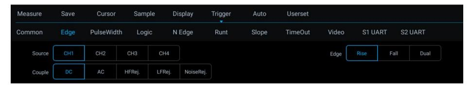
Figure 6-12 Edge Trigger Setting Menu
