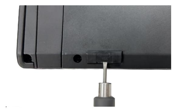
Figure 7-37 Opening the Fuse Protection Cover
