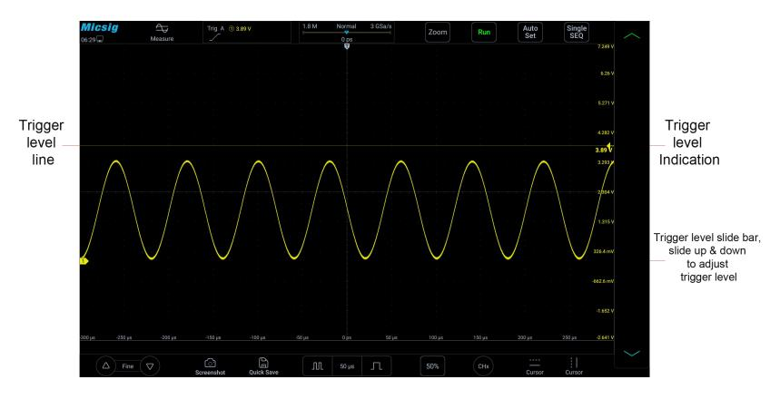
Figure 6-8 Trigger Level
