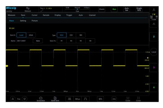
Figure 8-5 Save CH1 Reference Waveform Interface
