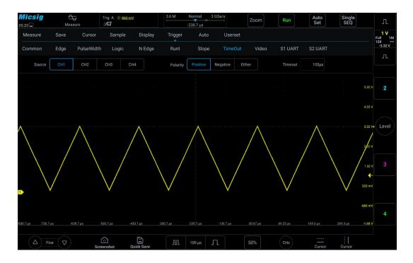
Figure 6-29 Time-out Trigger
