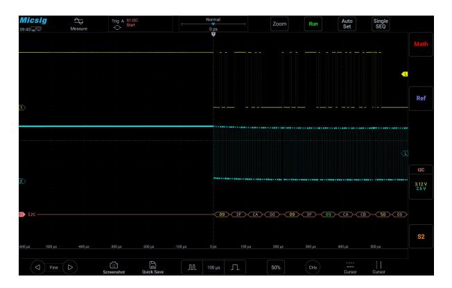
Figure 12-24 I<sup>2</sup>C Graphic Interface
