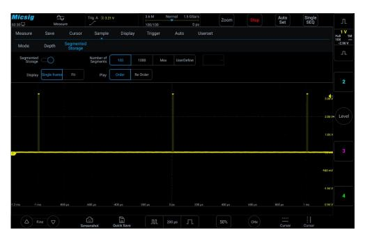
Figure 11-11 Segmented storage waveform acquisition
