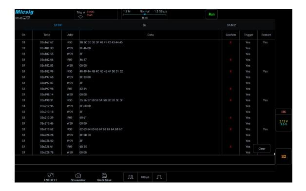
Figure 12-25 I<sup>2</sup>C Text Interface
