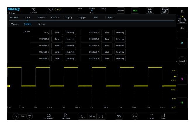
Figure 8-7 oscilloscope setting save
