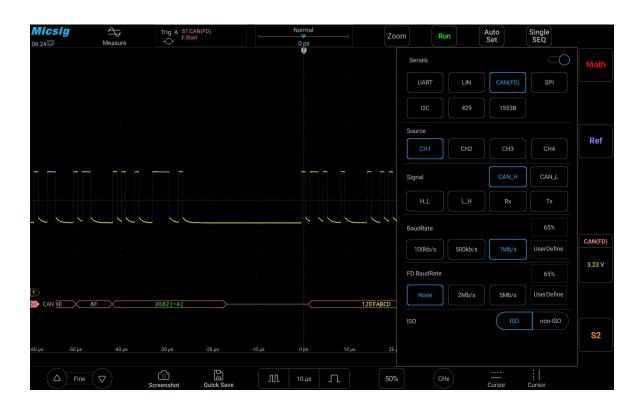
Figure 12-14 CAN / CAN FD Bus Configuration Menu
